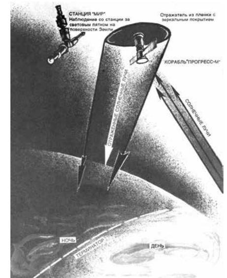
Fig. 1: Illumination scheme for Znamya 2. Once in space the device would unfurl a 20-metre-long spanning mirror that would deflect sunlight back to a nightbound area of the Earth.
